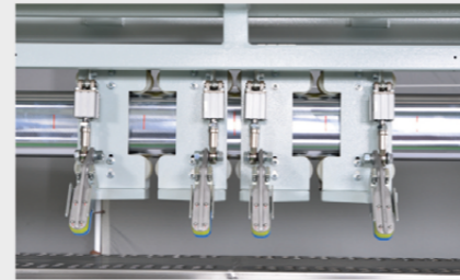
There are two set of feeding clamps, there must be one set feeding clamps waiting for an operator.
