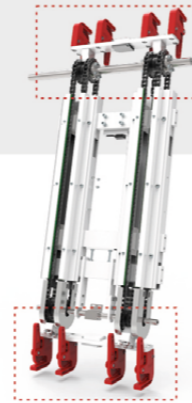
Two sets cycling of feeding clamps enhance the feeding efficiency.
